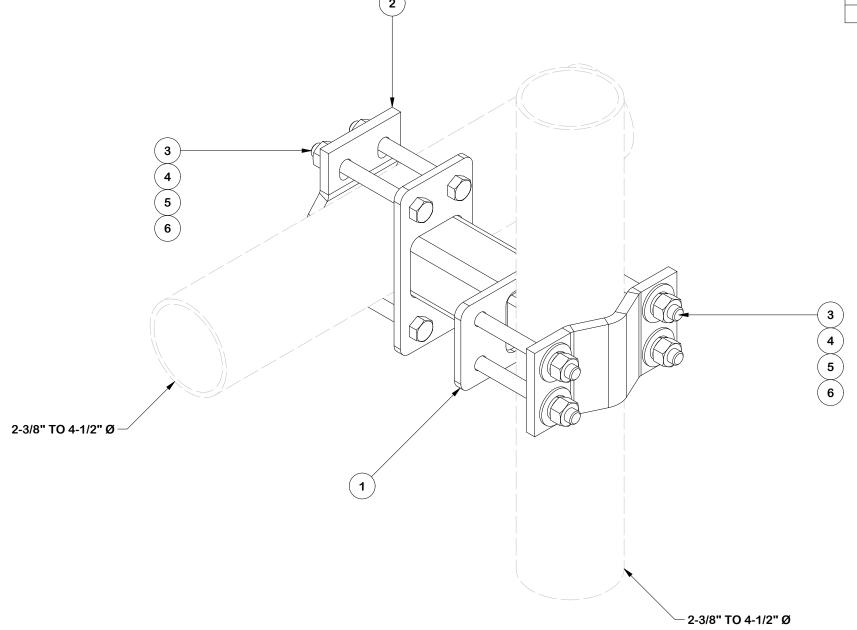
**PARTS LIST** ITEM QTY PART NO. PART DESCRIPTION LENGTH UNIT WT. NET WT. X-SOCX6 **6" STANDOFF CROSSOVER WELDMENT** 9.97 9.97 2 2 **V-CLAMP LARGE V-CLAMP** 8 21/32 in 5.55 11.09 3 8 G5806 5/8" x 6" HDG HEX BOLT GR5 FULL THREAD 6 in 0.62 4.94 5/8" HDG USS FLATWASHER 4 G58FW 1/8 in 0.07 0.56 5 8 G58LW 5/8" HDG LOCKWASHER 0.03 0.21 5/8" HDG HEAVY 2H HEX NUT **G58NUT** 0.13 1.04 TOTAL WT.# 27.81
